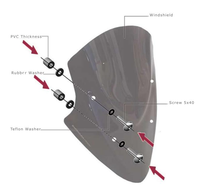
REMOVE THE 4 FIXING SCREWS OF THE ORIGINAL WINSHIELD, MOUNT THE BARRACUDA WINDSHIELD/SCREEEN WITH THE SPECIFIC THICKNESS LIKE DESCRIBED UP.
